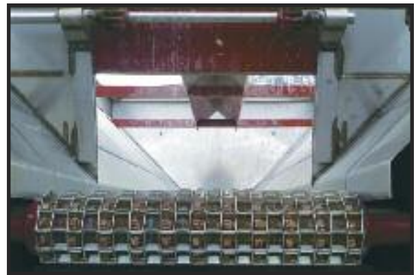
Be sure to adjust the door height based on the application rate and the spreader's ground speed.
